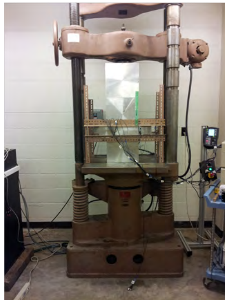
FIG. 3. Aluminum samples inside the Instron 100 klbs load frame. The bottom two blocks form the geometry of Figure 1, and the top block is used as a spacer to help distribute load evenly along the surface. The transducer frame can be seen holding the array platen on the left side of the blocks.
