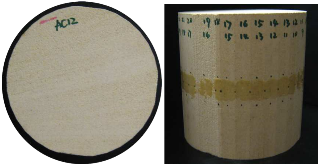
(a) Top view of AC12 showing the fine layering in the sample. (b) Side view of AC12 showing machined flats.
